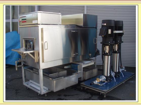
MU Series automatic fish-scale remover completely eliminates manual scaling work in process of fish. Operators' job is only to feed fish to conveyer of the machine and pick up scaled fish. The machine automatically and efficiently removes scales with high pressure jet water. Line speed and water pressure can be adjusted by very simple operation to make the optimum condition for processed fish. Rotating mesh belt screens removed scales from water so as to keep the circulated water clean.
