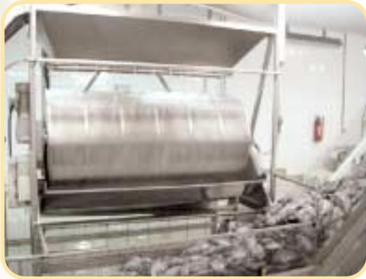
The DS-series drum scaling machines scale the fish by gently spinning them in a metal mesh drum. The rotating action and friction between the fish and the mesh removes the scales. The fish are scaled for a predetermined length of time controlled by an automatic adjustable timer. This ensures that the fish are scaled without any damage to the eyes or gill plate.
