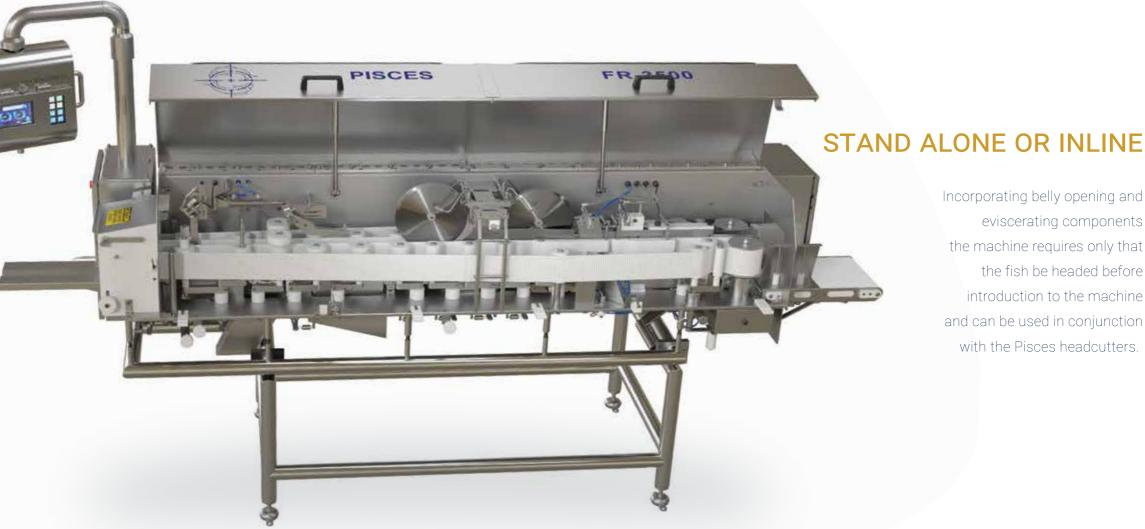
Incorporating belly opening and eviscerating components the machine requires only that the fish be headed before introduction to the machine and can be used in conjunction with the Pisces headcutters.
