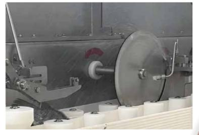
SPECIFICALLY DESIGNED TO PRODUCE HIGH-YIELD FILLETS FROM FISH IN THE SIZE RANGE 600 G TO 3.5 KG DEPENDING ON SPECIES. THROUGHPUTS UP TO 30 FISH / MINUTE DEPENDING ON FISH SIZE.
