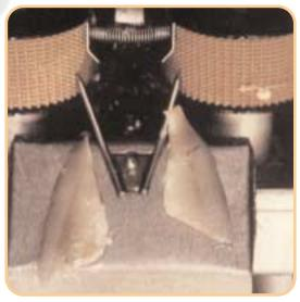
The Pisces FR-150 and FR-200 are reliable, versatile, high-speed filleting units specially designed for the production of single fillets free of backbone and ribs. Only minor adjustments are required to process a wide variety of fish species and sizes due to the machines' unique location method that utilizes the internal bone structure of the fish.
