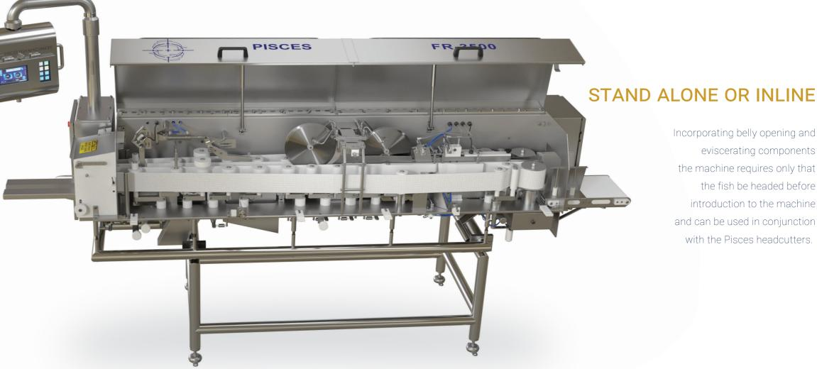
Incorporating belly opening and eviscerating components the machine requires only that the fish be headed before introduction to the machine and can be used in conjunction with the Pisces headcutters.
