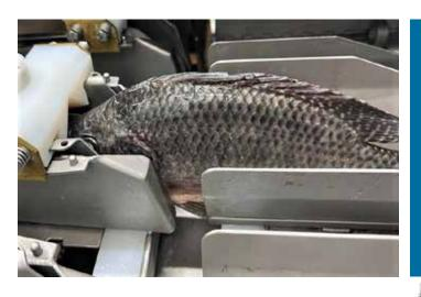
**SPECIFICALLY DESIGNED** TO PRODUCE HIGH-YIELD, HIGH SPEED HEAD REMOVAL FROM FISH IN THE SIZE RANGE HS-10 FROM 113 G TO 454 G HS-20/HV-25/30 FROM 340 G TO 2.7 KG HV-40 FROM 2 Kg TO 10 Kg.
